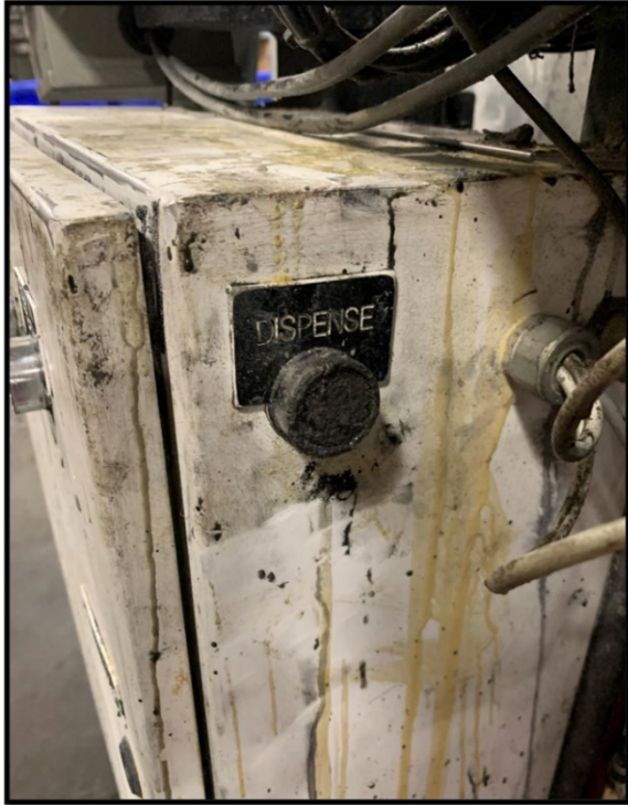
Figure #12 Dispense Machine Inside the air solenoids operate the Inject Slide and Purge Tube. With safety disabled, the solenoids move the plunger, pushing the chemical through the TAH head and out of the mixing block.
